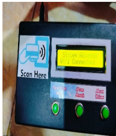
Fig. 5 IoT-Based Attendance Device
